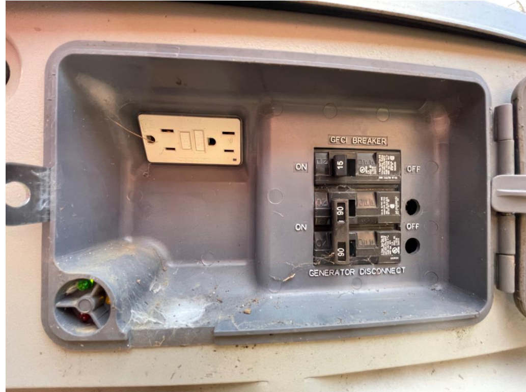
OUTPUT CB, 110 V UTILITY RECEPTACLE STATUS LED's (lower-left)
